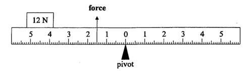
What upward force must be exerted at a point 1.5 meters from the pivot, as shown above, in order to just support the box?
